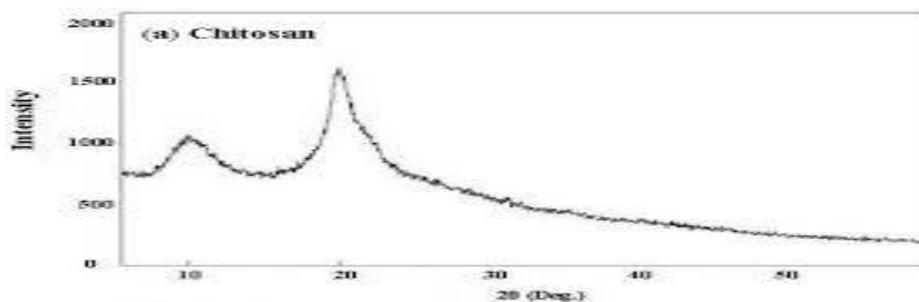
Fig-(4): X-ray diffractogram of pure chitosan
