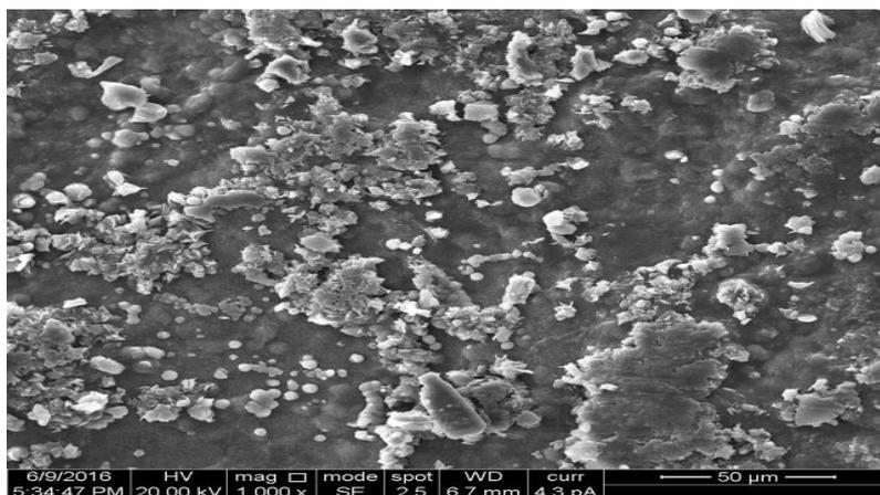
**Fig-(7):** SEM image of chitosan-o-Vanillin schiff base/ Polypropylene glycol blend
