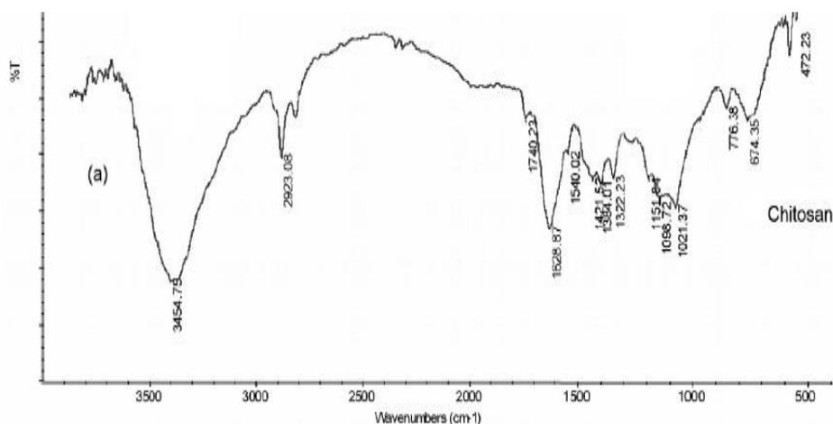
**Fig-(1): FT-IR spectrum of pure chitosan**
