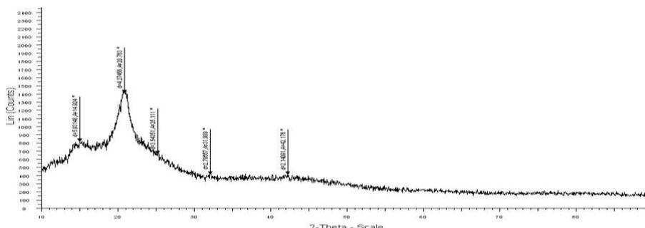
Fig-(5): X-ray diffractogram of chitosan – o-vanillin schiff base / Polypropylene glycol blend
