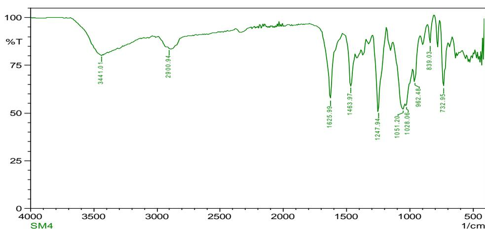
**Fig-(2): FT-IR spectrum of chitosan- o-Vanillin schiff base**
