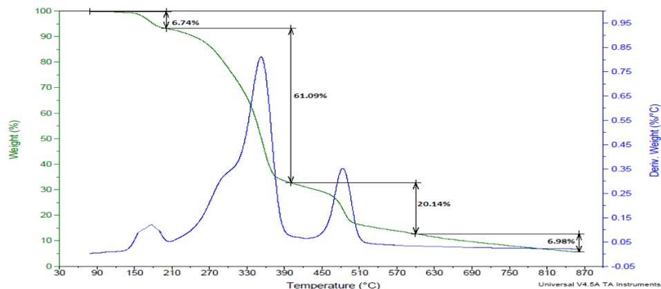
**Fig-(6):** TGA thermo gram of chitosan-o-vanillin/polypropylene glycol blend
